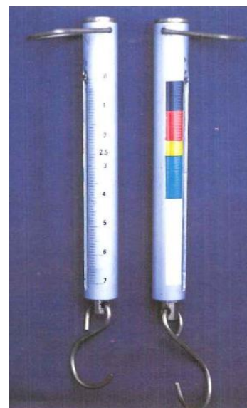
Figure 6. Coloured infant weighing scale, developed for the Tanjungsari study. 19
